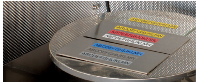
Fade resistant: after laminated labels were placed in a fade-inducing chamber to simulate a year in sunny surroundings, the text was unaffected
