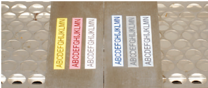
Temperature resistant: laminated labels text was found to be unaffected under extreme environment.
