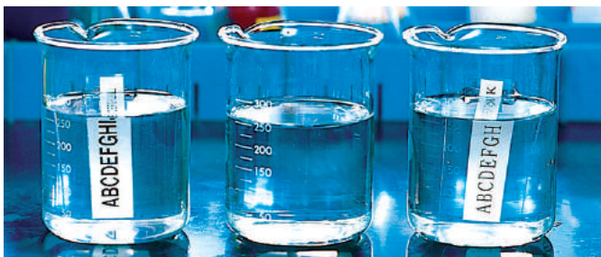
Water and chemical resistant: glass plates with laminated labels attached were immersed in water and various chemicals for two hours. The text was unaffected
