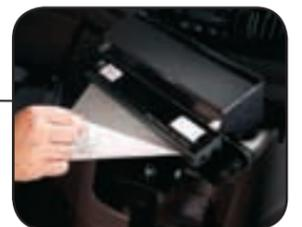
Use A4 cut sheet paper or continuous paper rolls - simply tear the paper once printed
